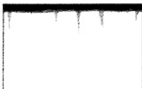
Figure 3.7.3.5 Microscopic evaluation at 200x of some thermal fatigue cracks developed in samples (Figure 3.7.3.4) from the EWK/Thyssen Krupp Specialty Steel thermal fatigue test (Figure 3.7.3.3) (Ref. 68)
